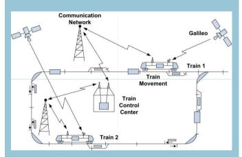
The objective of the GaLoROI project is the development of a certifiable safety relevant satellite based on-board train localisation unit to be used on low traffic density railway lines.
